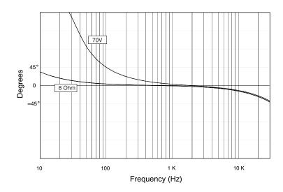
Figure 7.3 CTs 8200 Typical Frequency Response (1 W)
